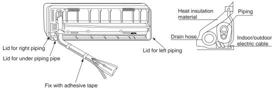
• Indoor/outdoor electric cable and drain hose must be bound with refrigerant piping by protecting tape.
